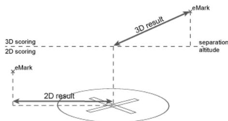
When goals/targets above the ground are used, results based on track points will be the 3D-distance.
